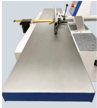
3,000 mm long, longitudinally profiled cast iron tables, each measuring 1,500 mm
