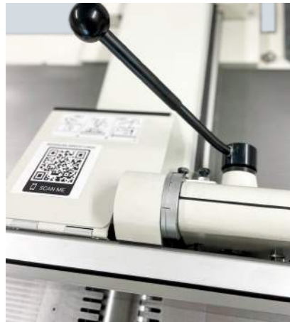
Fence adjustment via one-hand operation with angle display
