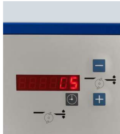
Electric depth adjustment accurate to 0.1 mm with the option to switch to an hour meter
