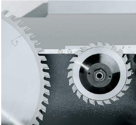
The scorer. Seperate 0.37 kW scoring motor with on/off switch.
